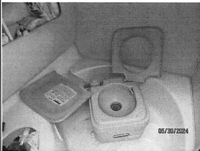
Toilet lid and seat broke at hinge
