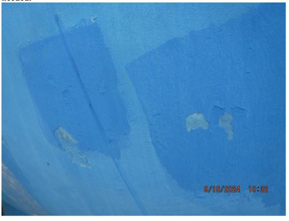
4- The rudder shows signs of moisture intrusion at 72%. Address as needed.
