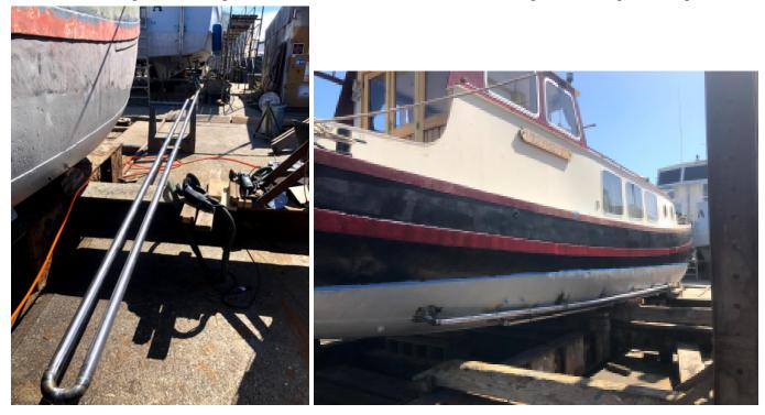
Engine oil is cooled by a inline cooler on the return of the keel cooler and a hand operated pump on the aft of the engine can be used to remove oil from the engine.
