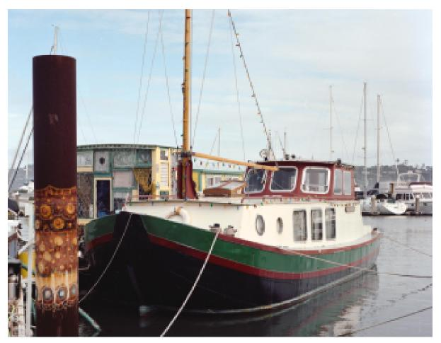
Vreyheyt II is a 37 foot Dutch river barge built in 1920 in the Netherland. Her hull is constructed of riveted iron sheets and has a Mercedes OM617 5 cylinder diesel for propulsion. She is fully navigable and has a modern solar and electrical system.
