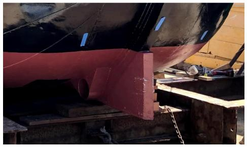
The vessel has a "Side Power" 12v bow thruster located in a tube in the "log splitter" with the head of the unit just forward of the waste water tanks under the bow locker and is powered by the lithium house batteries with heavy gauge cables run beneath the center of the cabin. The controller is a push-button type on the helm and the bow thruster can be isolated with a disconnect located by the main bus bar in the engine room.
