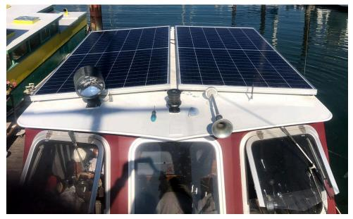
Two Canadian Solar 340W solar panels are installed on the roof of the wheel house and are connected to a Victron MPPT Solar Charger providing power to the house batteries. This system is capable of providing up to 5kWh during the summer.
