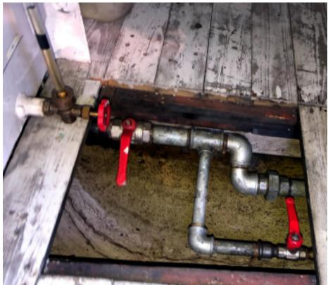
One *120L* fuel tank is located on the port side of the engine room with a sight glass as means to indicate level. The fuel manifold is located beneath the floorboards and controls fuel to the engine and heater.
