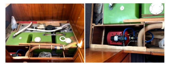
Two ~25 gal freshwater tanks are located under the main berth and can be filled via a deck port on the bow. Both tanks supply a pump and accumulator behind the tanks to port, and which distributes to the head, galley, and water heater via brazed copper pipe. Water was heated with a propane heater located in the head.
