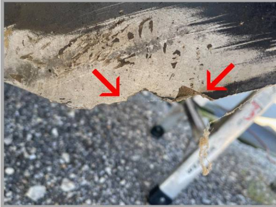
damaged outdrive skeg
