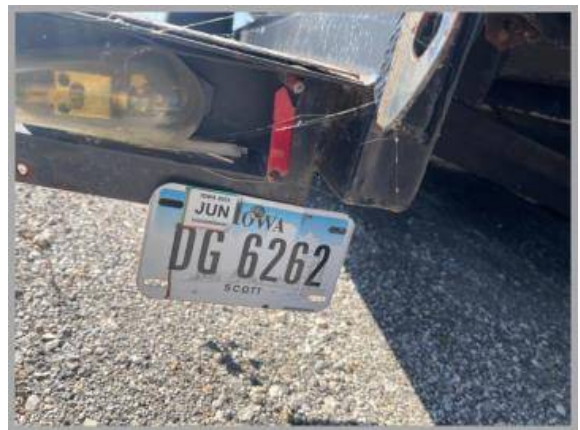
left tail light lens broken
