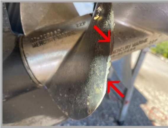
damaged prop blades
