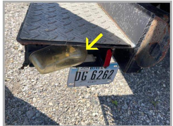
left tail light lens broken
