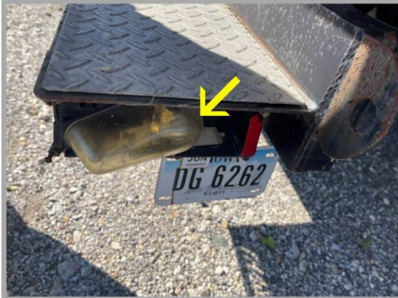
left tail light lens broken
