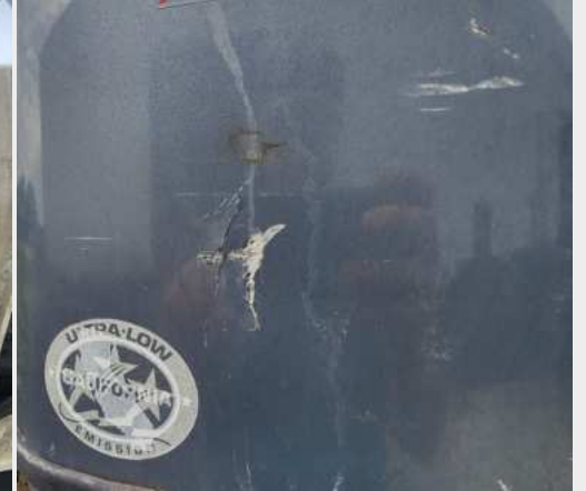
Minor corrosion and dirty was observed at the base of the power head. 1x aftermarket trim and tilt system operates properly. 1x transom anode of cut off. 1x engine cowling is cracked through on the aft side.
