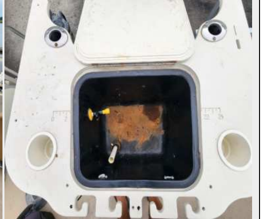
1x portside storage compartment is functional. 1x aft storage compartment lift supports are broken. 1x aft livewell is in sound condition but does not operate.
