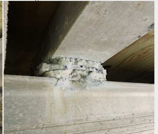
The marine grade plywood decks are sound with no evidence of saturation or rot from the underside. 4x aft pontoon engine support brackets are heavily corroded and bent.
