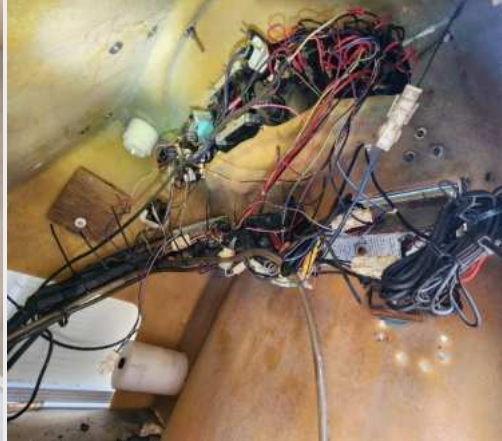
1x livewell in front of the helm console is structurally sound but not functional. The helm rigging is mostly organized and supported. FRP helm station is structurally sound and well-supported.
