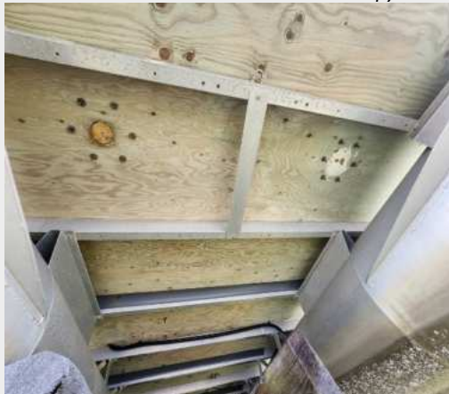
The marine grade plywood decks are sound with no evidence of saturation or rot from the underside. 4x aft pontoon engine support brackets are heavily corroded and bent.
