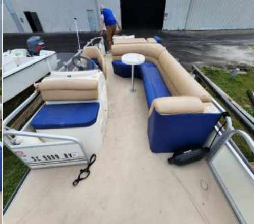
The marine plywood and vinyl foredeck, main deck, and aft deck, are structurally and cosmetically sound and well-supported.
