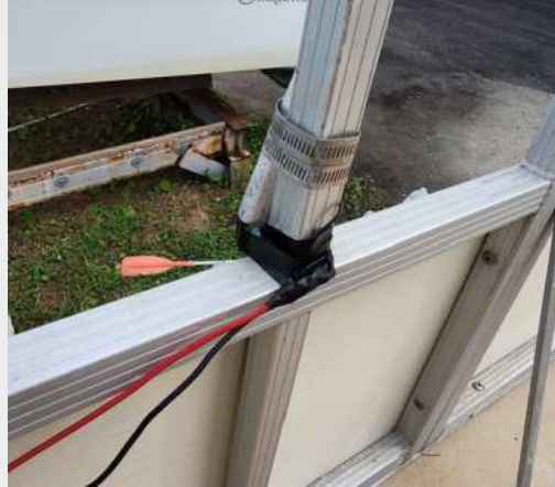
1x anchor light powers on but is mounted with tape and hose clamps. 2x bow casting chairs and mounts have been removed. 1x Danforth anchor and rode are in serviceable condition.
