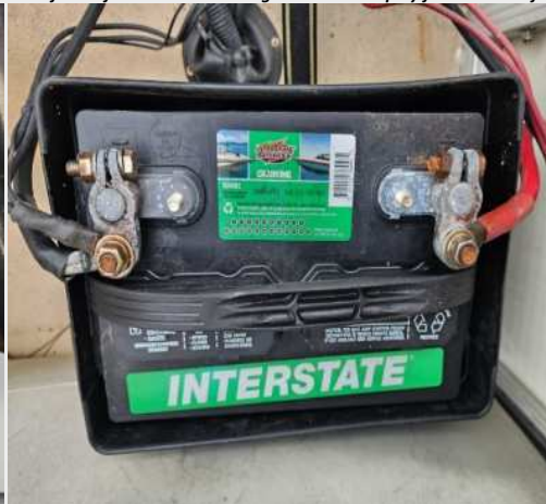
1x Cole Hersee battery switch is functional. 1x Interstate 24M-XHD battery in serviceable condition. 1x unverified manufacture livewell pump does not power on.
