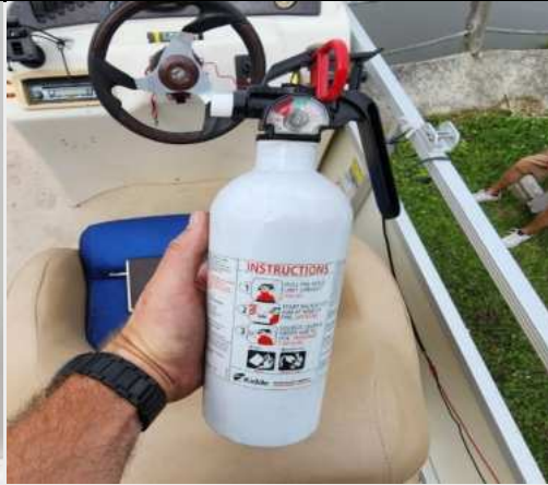
1x courtesy light on the side of the helm console does not power on. 1x Kidde fire extinguisher, 1x type-IV throwable & 8x type-II PFDs, in operational condition.
