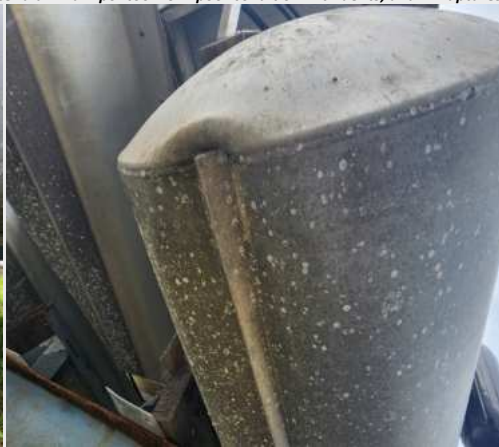
The starboard 25" diameter aluminum pontoon appears water tight but is dented, bent, and scratched.
