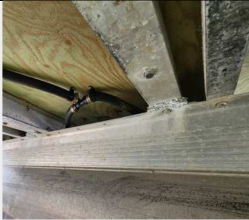
2x examples of the corrosion on the pontoon engine support brackets. 2x red and green nav lights power on. 2x bow docking lights do not power on.
