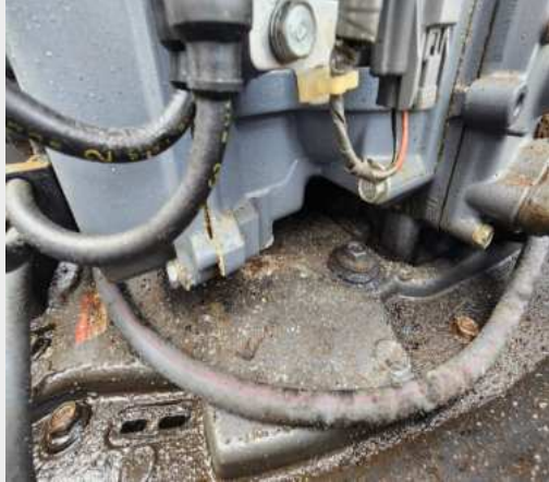
Minor corrosion and dirty was observed at the base of the power head. 1x aftermarket trim and tilt system operates properly. 1x transom anode of cut off. 1x engine cowling is cracked through on the aft side.
