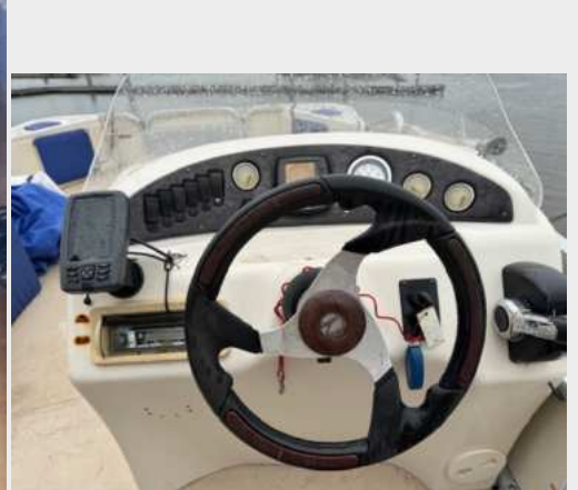
1x livewell in front of the helm console is structurally sound but not functional. The helm rigging is mostly organized and supported. FRP helm station is structurally sound and well-supported.
