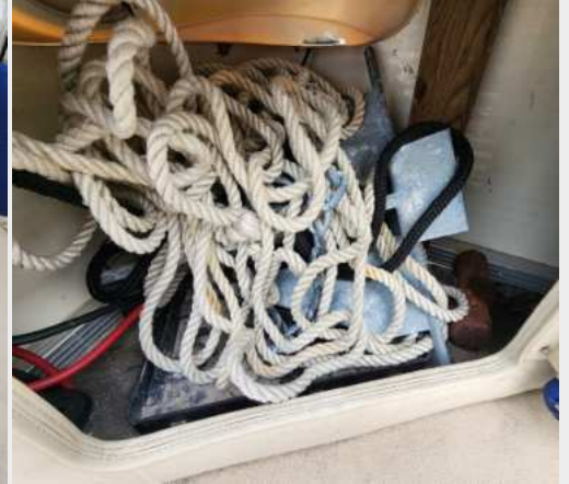
1x anchor light powers on but is mounted with tape and hose clamps. 2x bow casting chairs and mounts have been removed. 1x Danforth anchor and rode are in serviceable condition.
