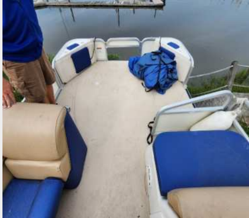
The marine plywood and vinyl foredeck, main deck, and aft deck, are structurally and cosmetically sound and well-supported.
