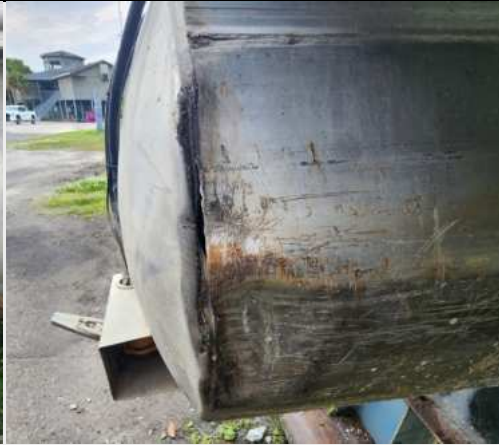
The port 25" diameter aluminum pontoon is in poor condition with dents, and 2x ruptures at the aft cap welds.
