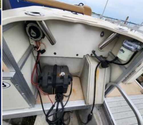
1x aft casting chair is not onboard. In front of the motor is 1x 31-gallon crosslink poly fuel tank and fuel filter in serviceable condition.
