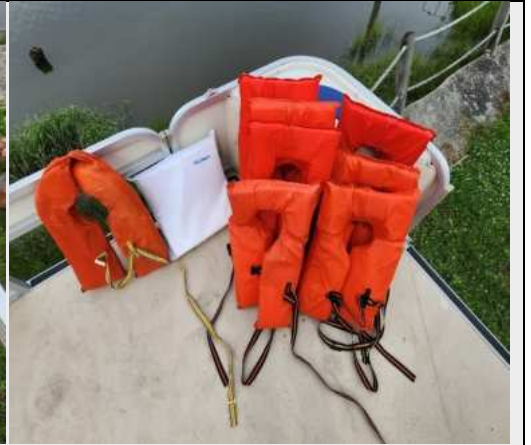
1x courtesy light on the side of the helm console does not power on. 1x Kidde fire extinguisher, 1x type-IV throwable & 8x type-II PFDs, in operational condition.
