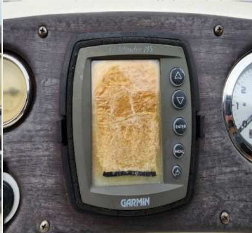
6x vessel control switch labels are difficult to read. 1x Garmin Fishfinder 85 does not operate. 1x Dual stereo does not function.
