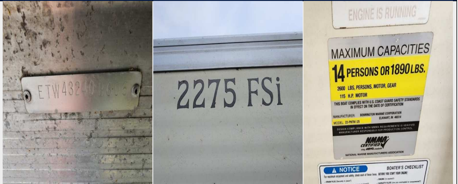
Hull identification number (HIN: ETW43240B606) & Bennington Pontoon model designator & capacities plate aboard the 2006 Bennington 2275 FSi
