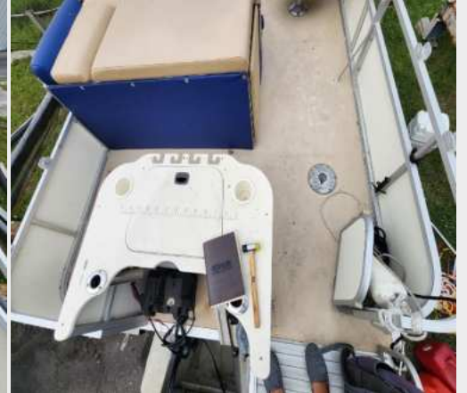
The marine plywood and vinyl foredeck, main deck, and aft deck, are structurally and cosmetically sound and well-supported.
