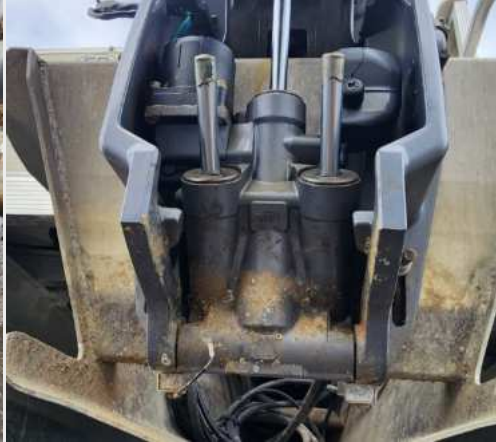
Minor corrosion and dirty was observed at the base of the power head. 1x aftermarket trim and tilt system operates properly. 1x transom anode of cut off. 1x engine cowling is cracked through on the aft side.
