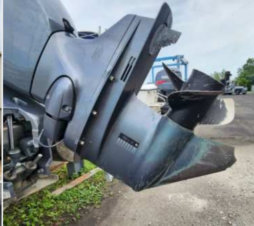
Cosmetic damage to the 1x engine cowling. 1x lower unit has cosmetic paint wear and scratches. 1x 3-blade propeller is damaged on the leading edge of each blade.
