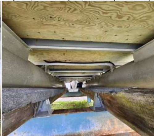
The marine grade plywood decks are sound with no evidence of saturation or rot from the underside. 4x aft pontoon engine support brackets are heavily corroded and bent.
