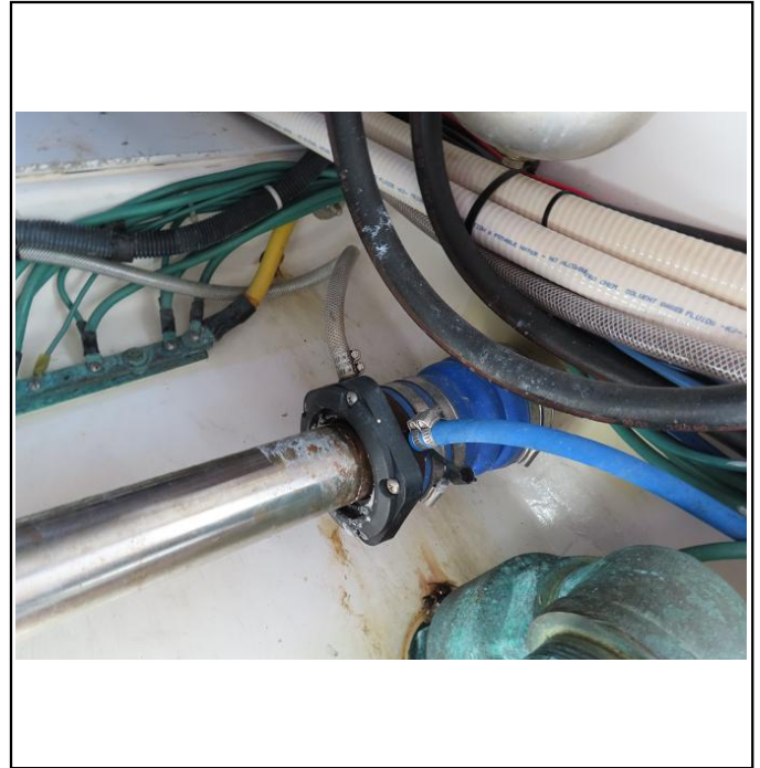
Starboard shaft seal
