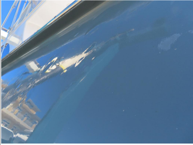
Hull sides blisters
