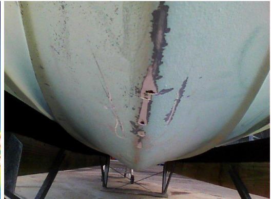
Under bow abraded section surface damage only.
