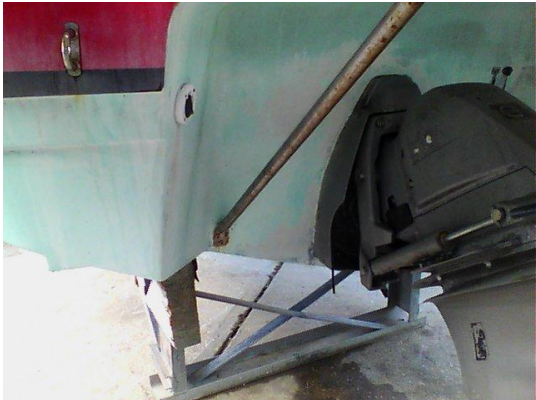
Transom with swim platform mounts and drive pass through no moisture or voids observed.
